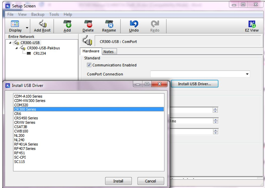
**FIGURE 3-2 INSTALLING THE USB DRIVERS WITHIN LOGGERNET™**
