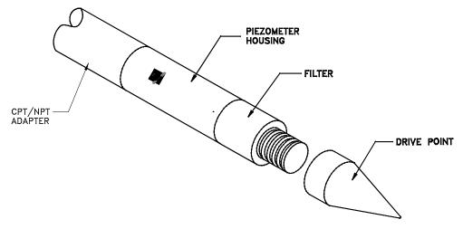
Figure 3 – Unscrew the drive point
