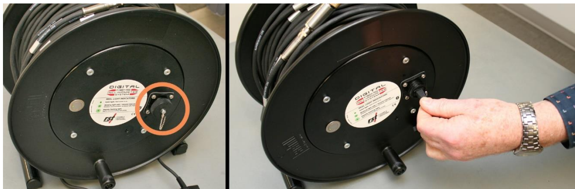
Figure 7 – Unscrewing the Battery Cap
