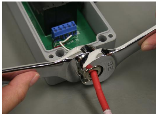
FIGURE 3-5 TIGHTENING THE CABLE GLAND
