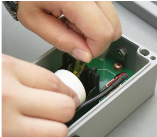
FIGURE 3-6 ACTIVATE THE BATTERY
