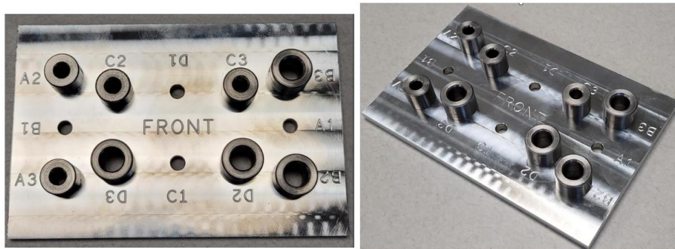
Figure 17: Concrete Drilling Template
