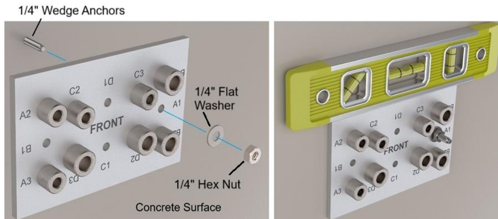
Figure 22: Leveling and Fastening Drilling Template on Hole A1 with 1/4" Wedge Anchor, Nut and Washer
