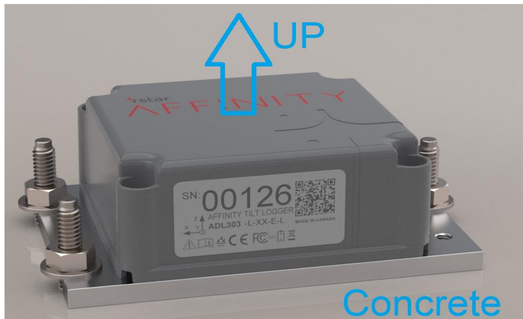
Figure 28: Direct Mounted Affinity Tilt Logger installed at Horizontal Orientation using 1/4" Wedge Anchors
