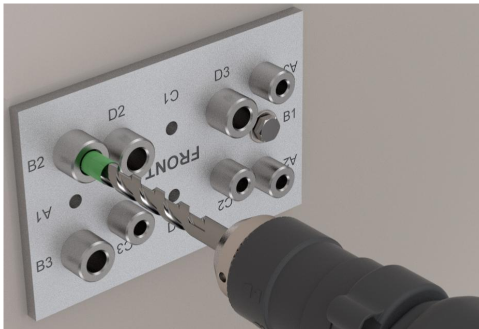
Figure 35: Drilling Second Hole Through Bushing B2 for Drop-In Anchor
