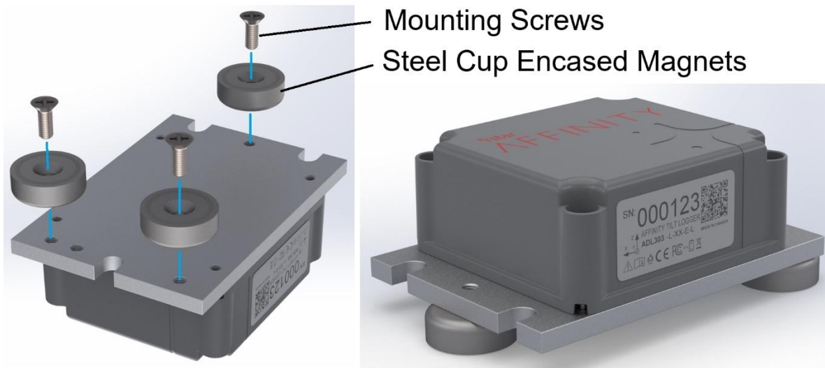
Figure 66: Installing Steel Cup Enclosed Magnets onto the Affinity Tilt Logger
