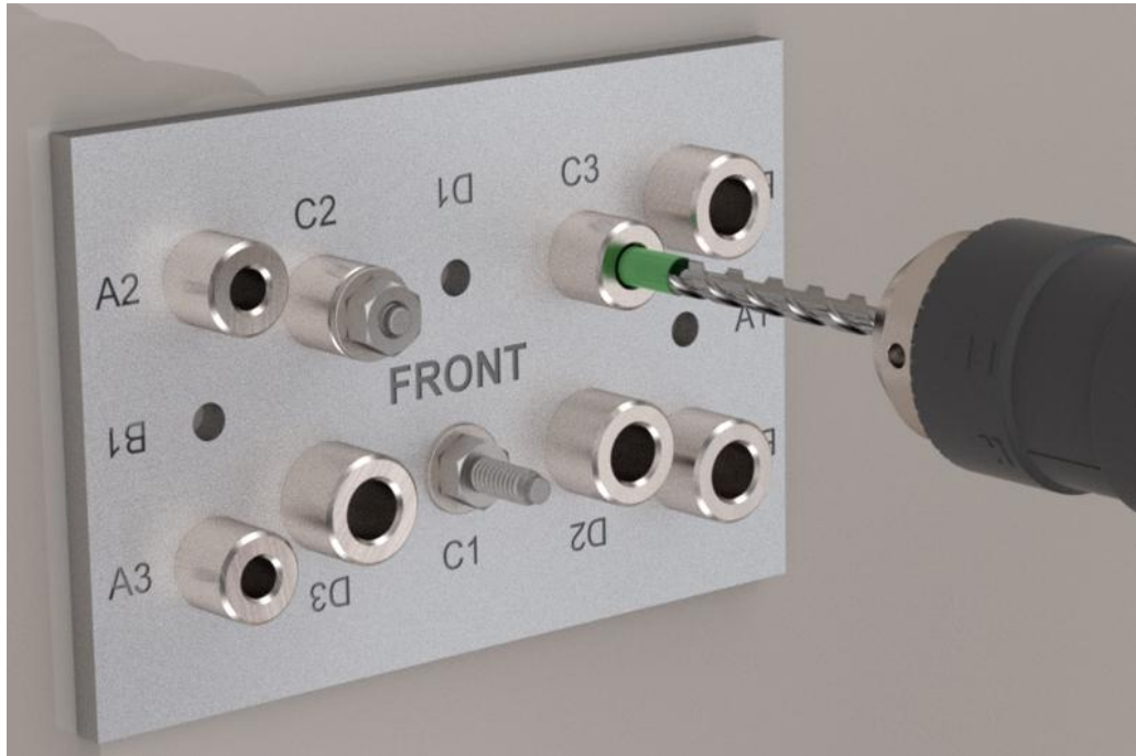
Figure 48: Drilling Third Hole Through Bushing C3 for Wedge Anchor
