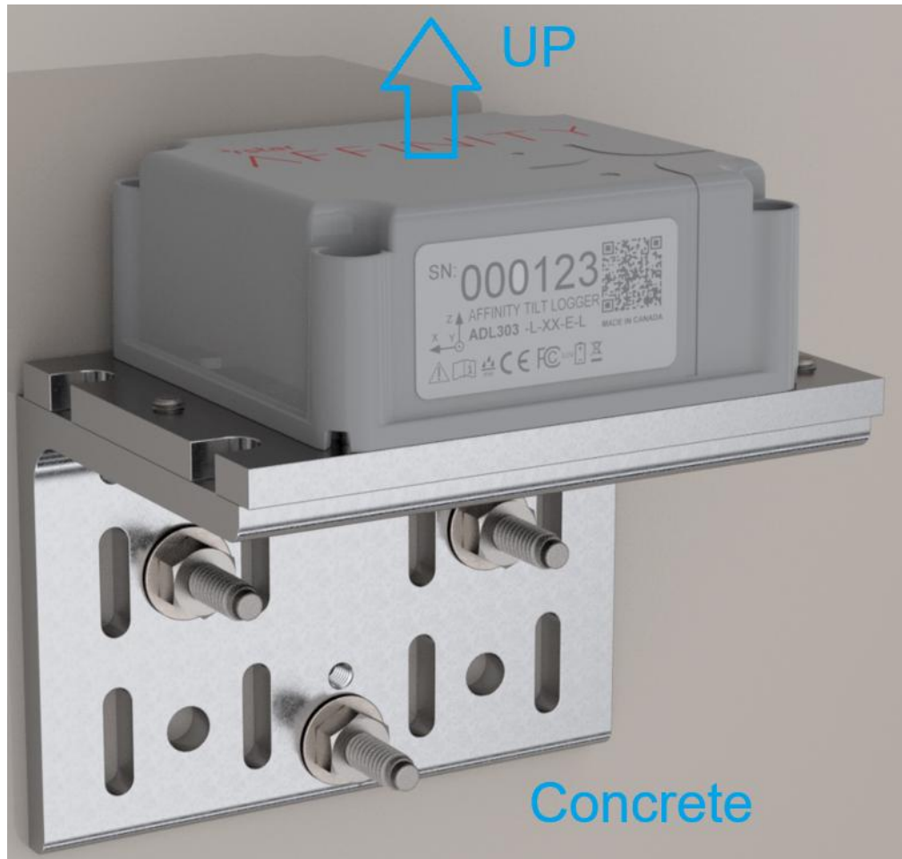
Figure 51: Angle Bracket Mounted Affinity Tilt Logger Installed in Horizontal Orientation Using 1/4" Wedge Anchors
