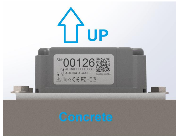
Figure 12: Direct Mounted Tilt Logger in Horizontal Orientation
