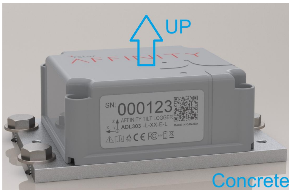
Figure 39: Direct Mounted Affinity Tilt Logger Installed in Horizontal Orientation Using 1/4" Drop-In Anchors
