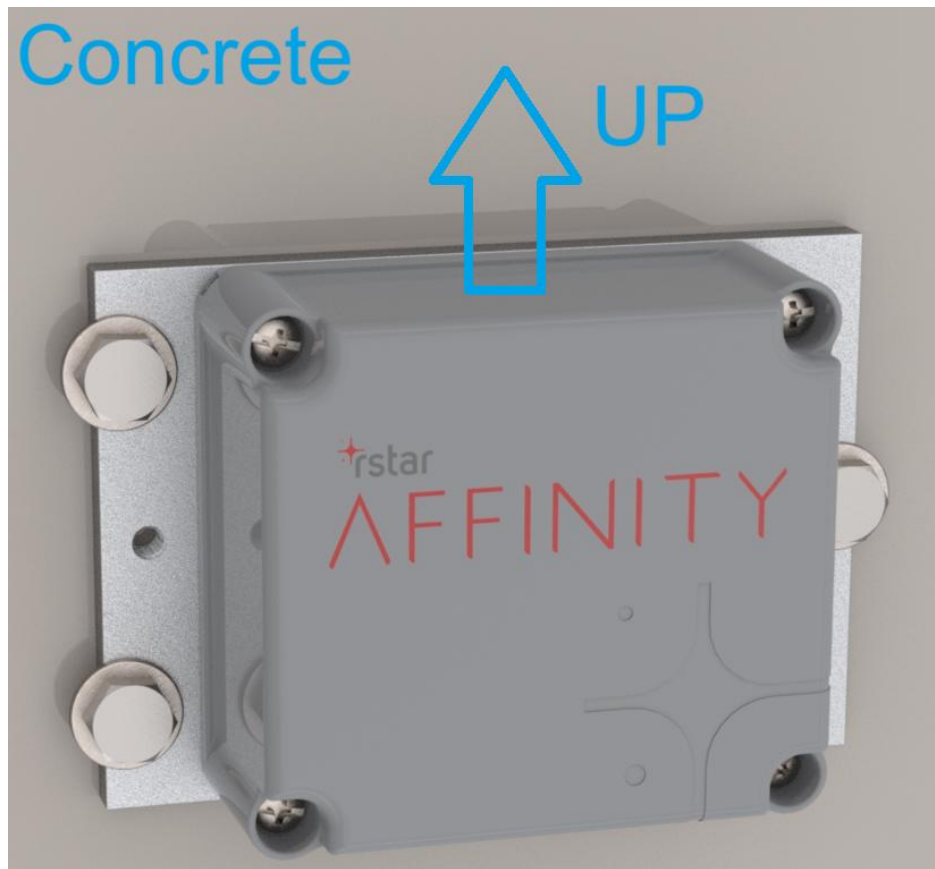
Figure 40: Direct Mounted Affinity Tilt Logger Installed in Vertical Orientation Using ¼” Drop-In Anchors
