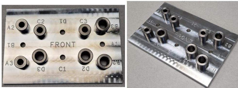
Figure 17: Concrete Drilling Template
