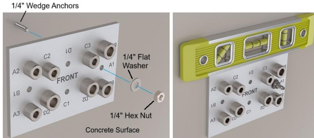
Figure 22: Leveling and Fastening Drilling Template on Hole A1 with 1/4" Wedge Anchor, Nut and Washer
