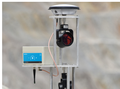
GMS700s can be used with NavStar's ACAL Advanced Calibration system for high precision prism monitoring.
