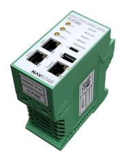
The FLP200 acts as a gateway with a high-speed processor, facilitating communication and data transfer between the GMS rover and GeoExplorer.
