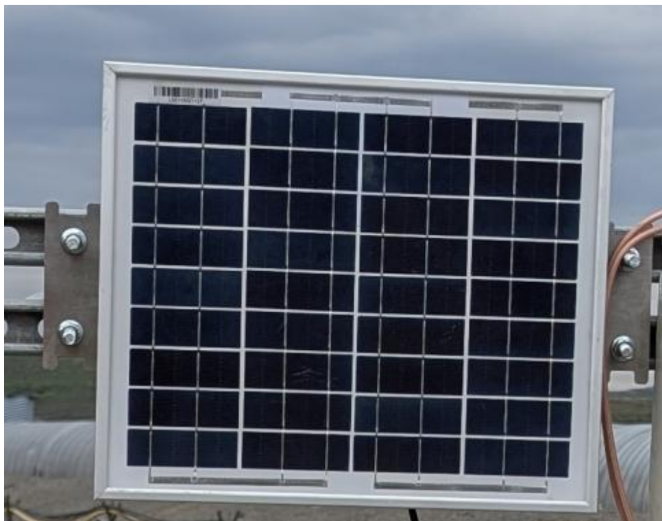
Figure 13: Solar Panel with Mounting Brackets and U-Bolts on Flat Surface/Stand
