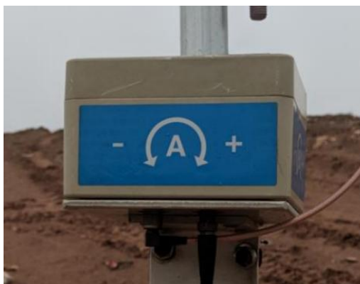
Figure 11: Example of GMS700 showing direction for Tiltmeter orientation
