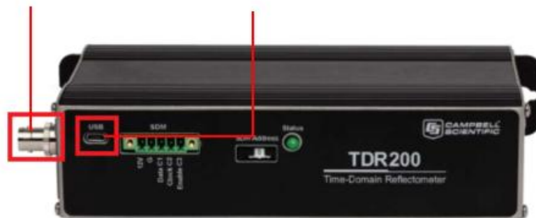
Figure 4: TDR200 Connections Overview
