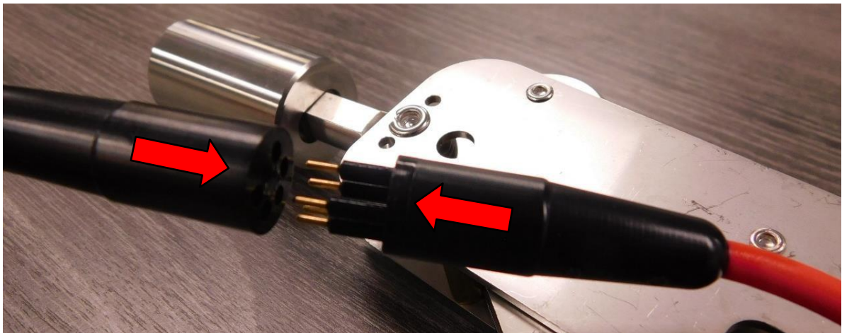
FIGURE 2-1 MATING THE CONNECTORS
