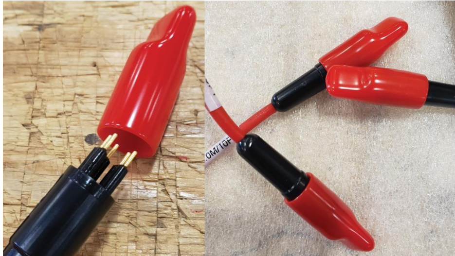
FIGURE 2-3 PLACE PROTECTIVE CAPS ON CONNECTORS WHEN NOT IN USE
