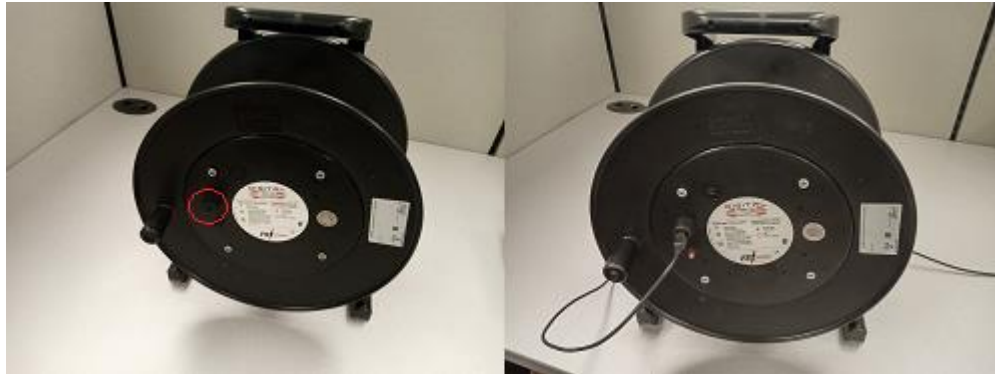
Figure 7 – Unscrewing the Battery Cap
