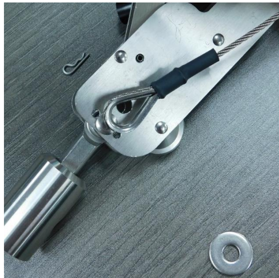
Figure 6: Place Safety Cable Against Bottom Wheel Assembly
