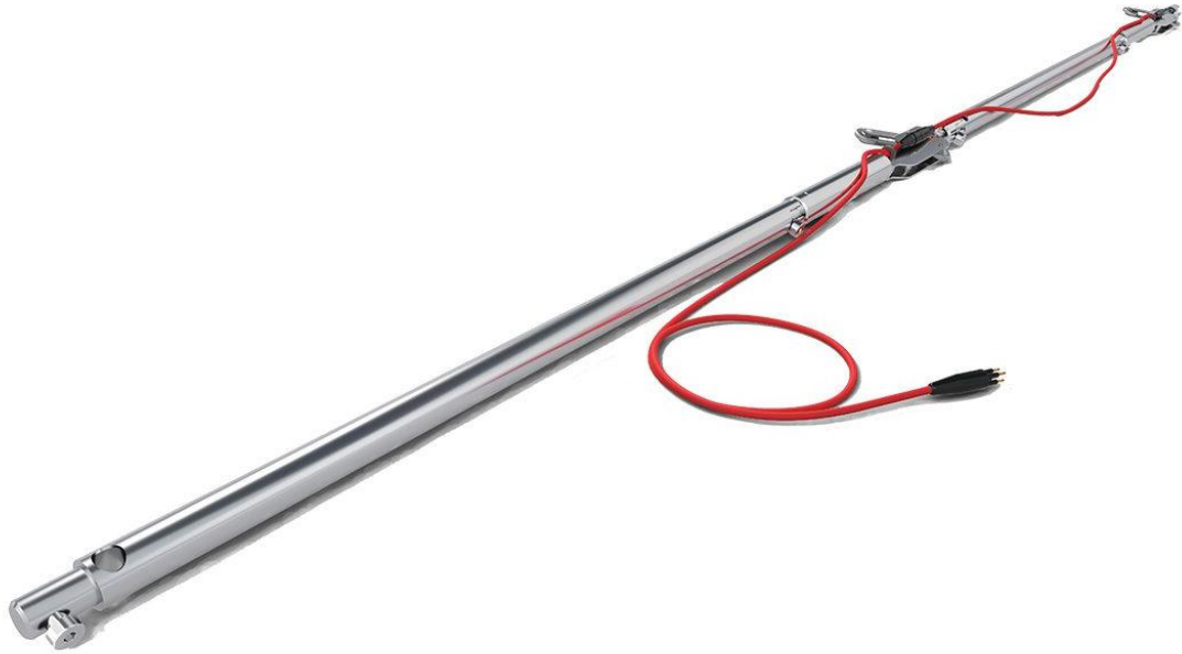
Figure 1: Overview of MEMS In-Place Inclinometer System
