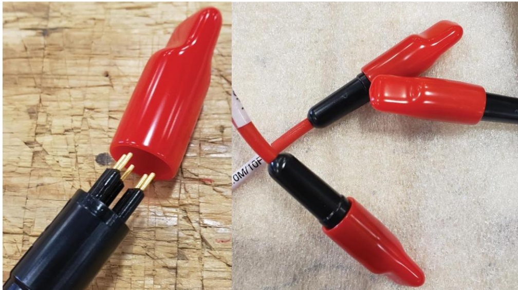
Figure 17: Protective Caps are Placed on the Connectors when not in use
