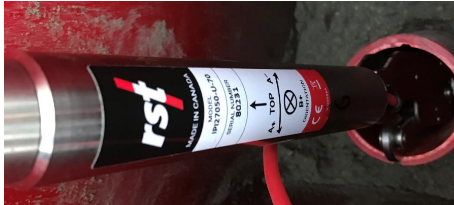
Figure 11: Lowering the Bay Assembly into the Inclinometer Casing
