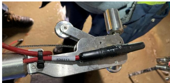
Figure 9: Attach the Bottom Plug onto the Bottom Sensor Cable
