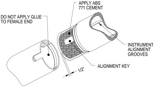
Figure 3 – Typical Casing Joint
