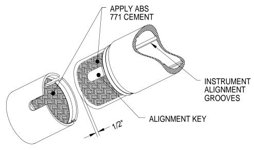
Figure 2 – End Cap Joint
