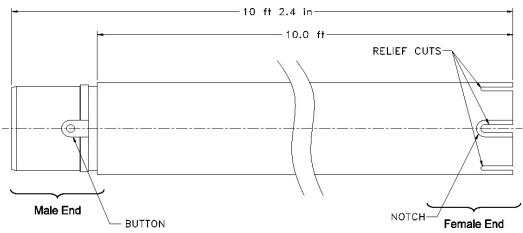
Figure 1 – RST Glue and Snap casing
