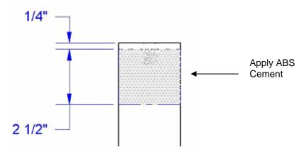
Figure 7 – Casing Preparation
