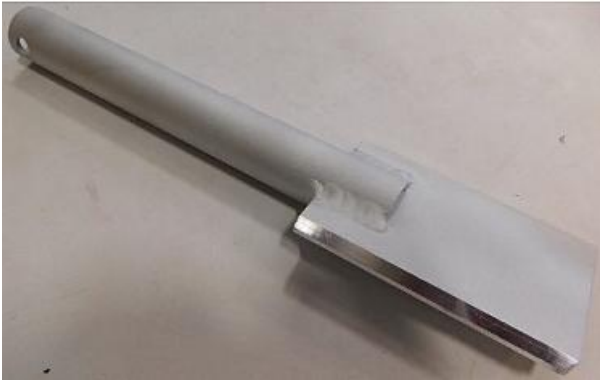
Figure 15: Casing Alignment Tool
