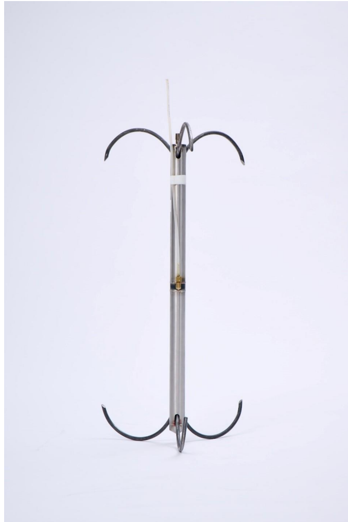
Figure 7: Borros Type Anchor Overview
