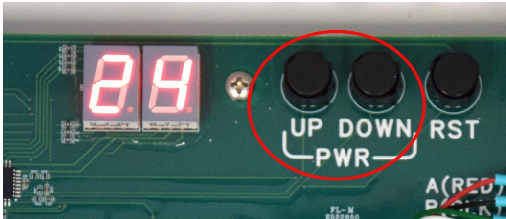
Figure 7: Up/Down Selection Button Detail
