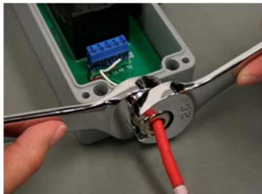
Figure 3-4 Tighten the cable gland
