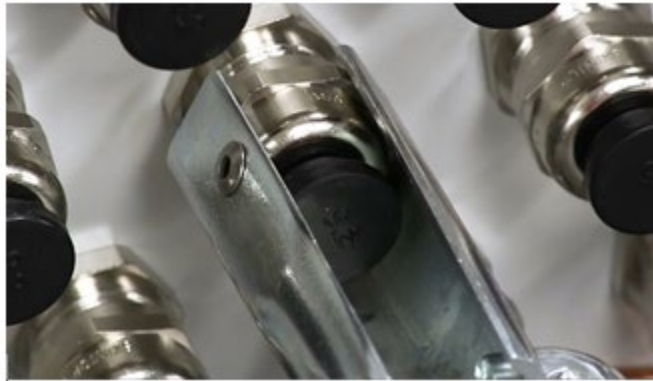
Figure 3-2 Loosen the cable gland using the cable gland nut wrench
