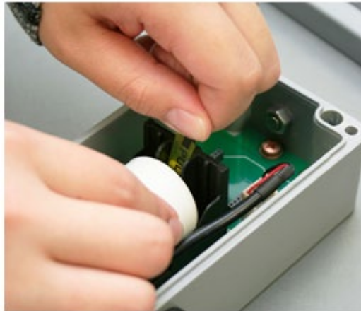
Figure 3-5 Activate the battery
