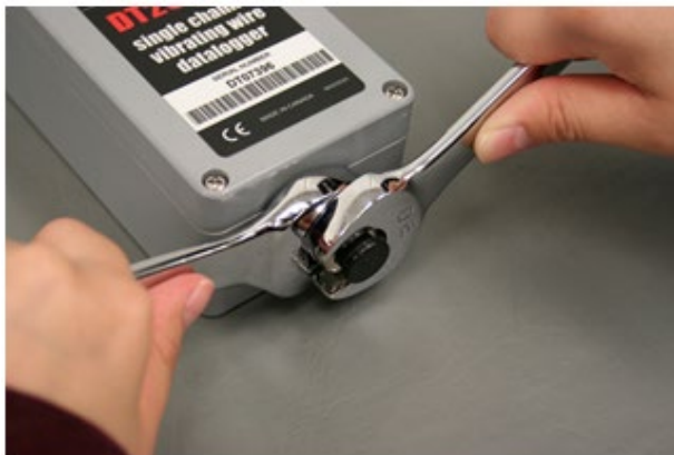
Figure 3-1 Loosen the cable gland using two 20 mm wrenches
