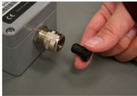
Figure 3-3 Remove the cable plug from the cable gland
