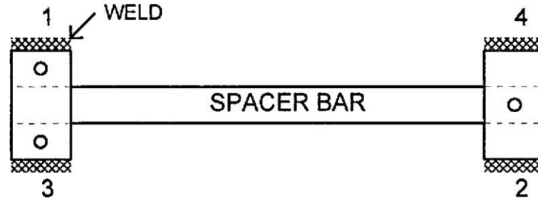
FIGURE 3-7 WELDING SEQUENCE FOR THE MOUNTING BLOCKS
