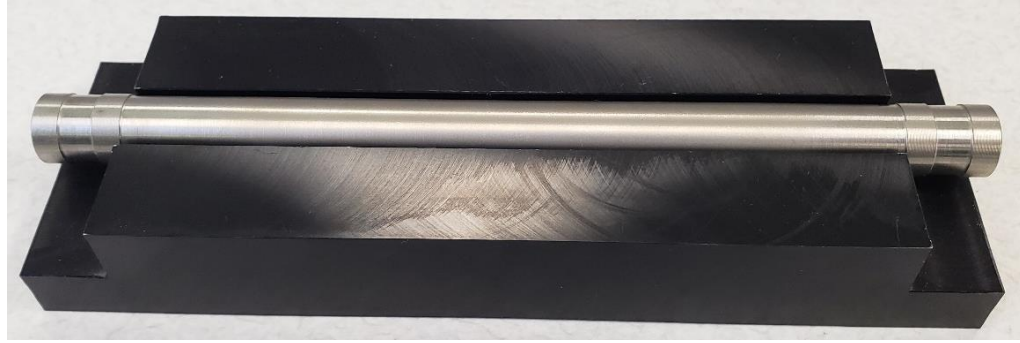
FIGURE 3-4 PLACE THE SPACER BAR ON THE SPACING JIG
