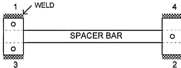
FIGURE 3-7 WELDING SEQUENCE FOR THE MOUNTING BLOCKS
