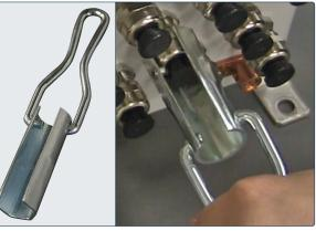
The Cable Gland Nut Wrench (DT100) improves access to the glands when compared to a standard wrench.
