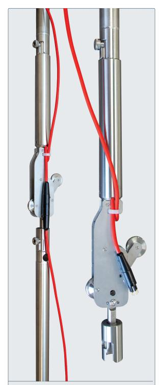
A close-up shows the signal cable which connects each sensor along the entire chain of inclinometer sensors forming a "digital bus"
