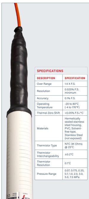
Corrosion Proof Vibrating Wire Piezometer
