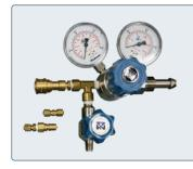
Inflation Regulators are used to control inflation of the borehole packers. Two models are available: 0-350 psi and 0-1500 psi. Each regulator includes a quick connect (to attach the packer inflation line) and a standard nitrogen bottle connector.
