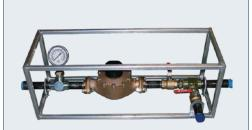
A Flow System is used to monitor and control water during downhole testing. Each flow system includes a flow meter, pressure gauge, shut-off valve, by-pass valve, connection hose, and aluminum frame.
