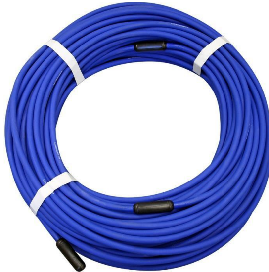
Figure 1: Thermistor String Coil Assembly
