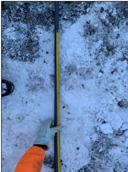
Figure 2: Measuring Thermistor String Length Required for Borehole Installation
