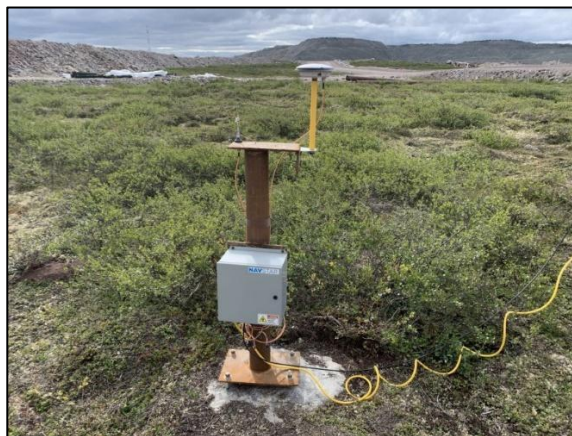
Figure 12: Example of GNSS Base Station Control Box Configuration Field Installation
