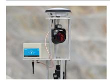
GMS800s can be used with NavStar's ACAL Advanced Calibration system for high precision prism monitoring.
