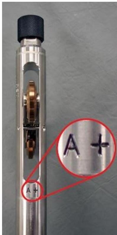
Figure 6: A+ Marking on the Inclinometer Probe to Determine Axial Orientation
