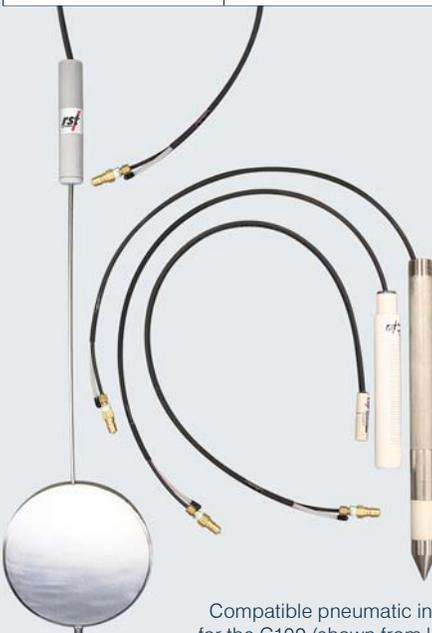
Compatible pneumatic instruments for the C109 (shown from left to right): Total Earth Pressure Cell, P-100 Mini Piezometer, P-100-1 Piezometer, and Pneumatic Wellpoint Piezometer.
