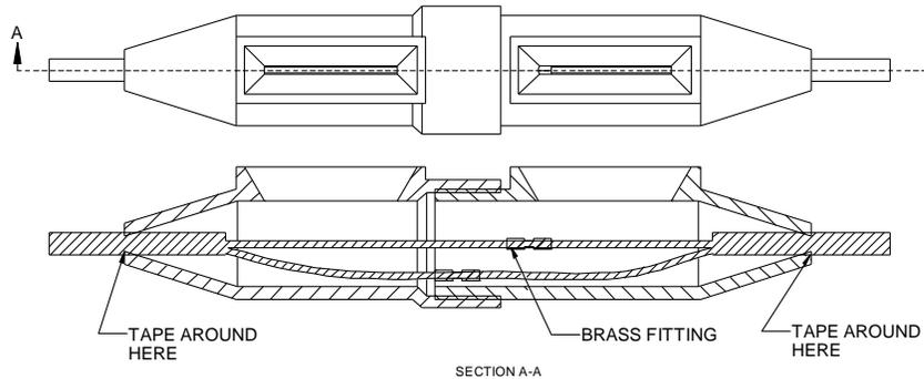
**Figure 2 – Splicing Pneumatic Tubing**
