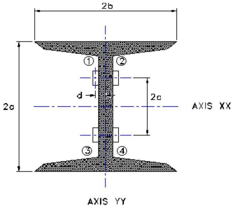
**Figure 7 - Strain Gauges Mounted on Central Web. Axial Strain and Bending Moments about both XX and YY Axes**
