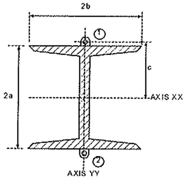
**Figure 10 - Axial Strain and Bending Moments about XX axis only**
