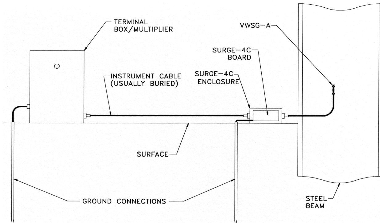
**Figure 6 - Lighting Protection Scheme**
