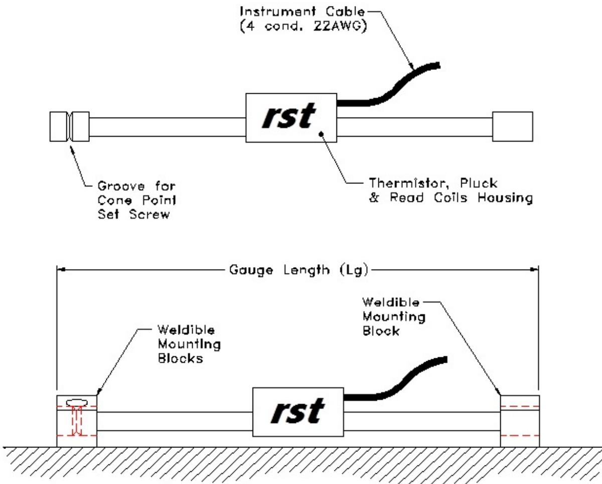
**Figure 1 - VWSG-A(M) General Arrangement**
