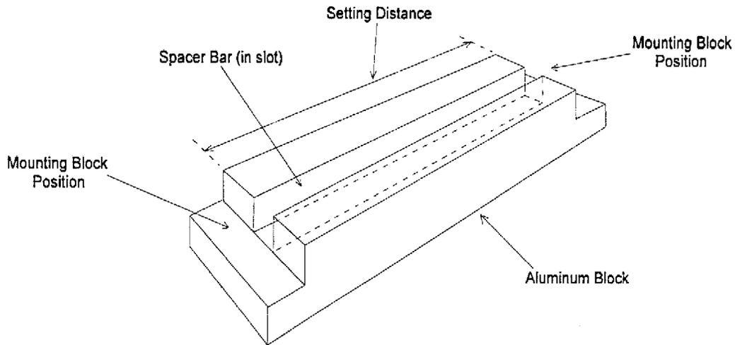
Figure 2 - Spacing Jig
