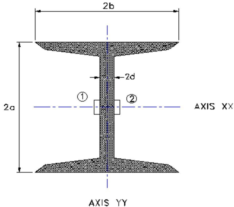
**Figure 9 - Axial Strain Measurement and Bending Moment about YY axis only**
