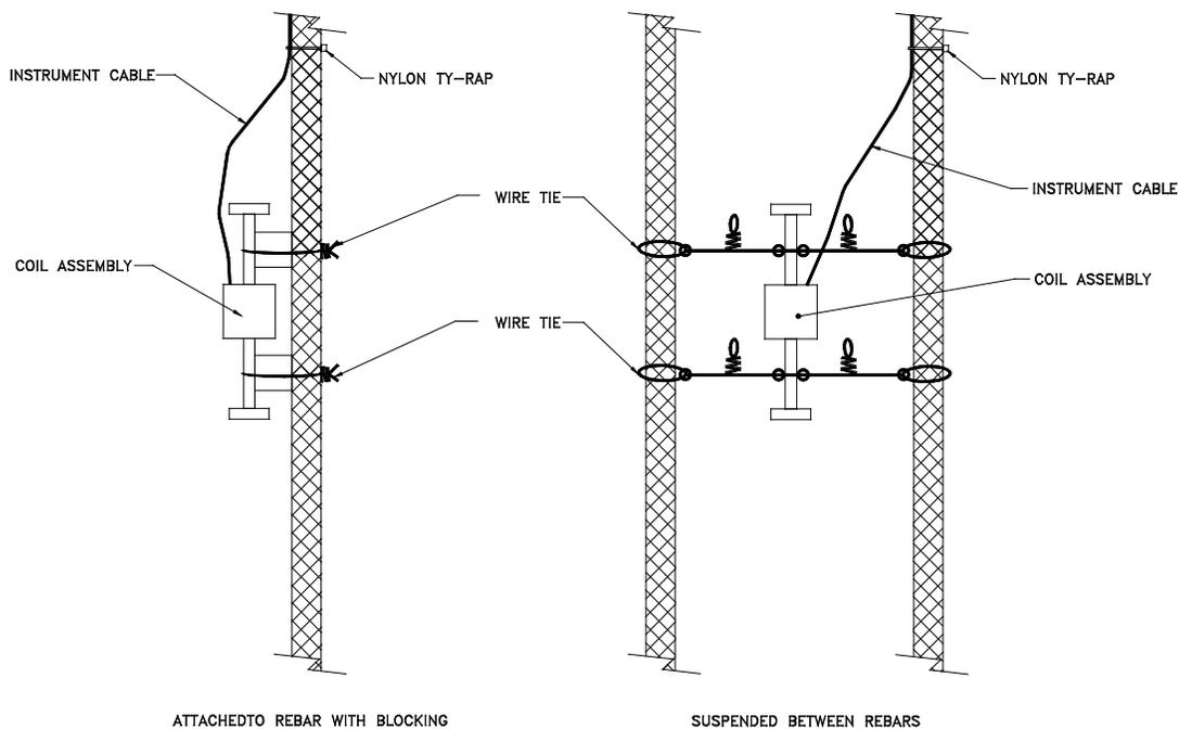
**Figure 5 – Attaching VWSG-E(M) Strain Gauges to Re-bar**
