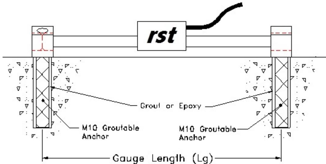
Figure 4 - Installation on Concrete using Groutable Anchors
