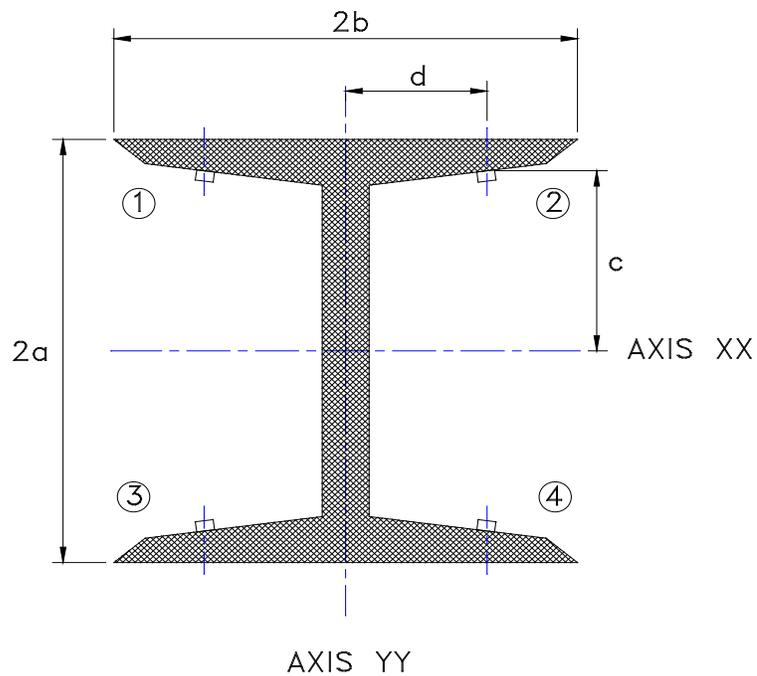
**Figure 8 - Strain Gauges Mounted on Flanges (Not Recommended)**
