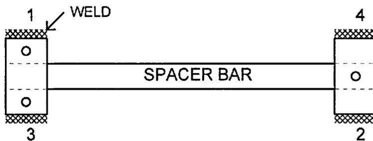
Figure 3 - Welding Sequence for the Mounting Blocks
