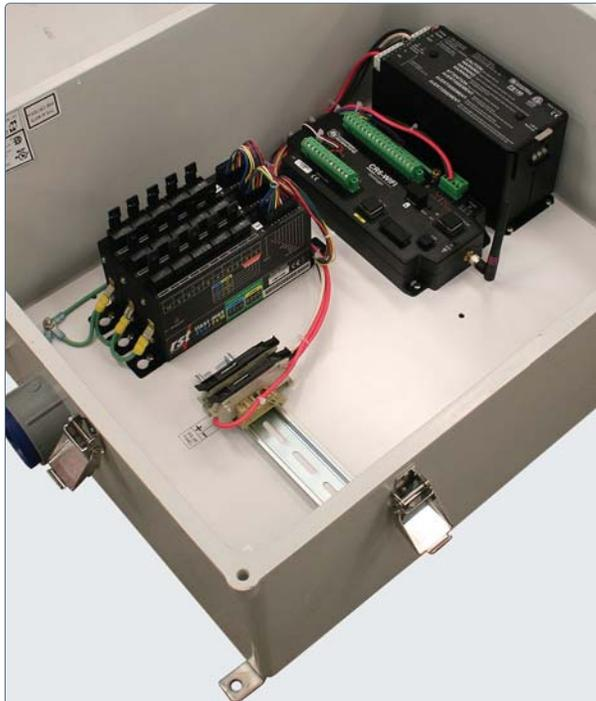
CR6 FlexDAQ Data Logger (with optional wi-fi) in a weatherproof enclosure with RST Flexi-Mux Multiplexers.
