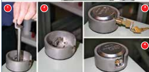
Logger Pedestal Enclosure with closeup of procedure for engaging vandal-resistant locking mechanism.
