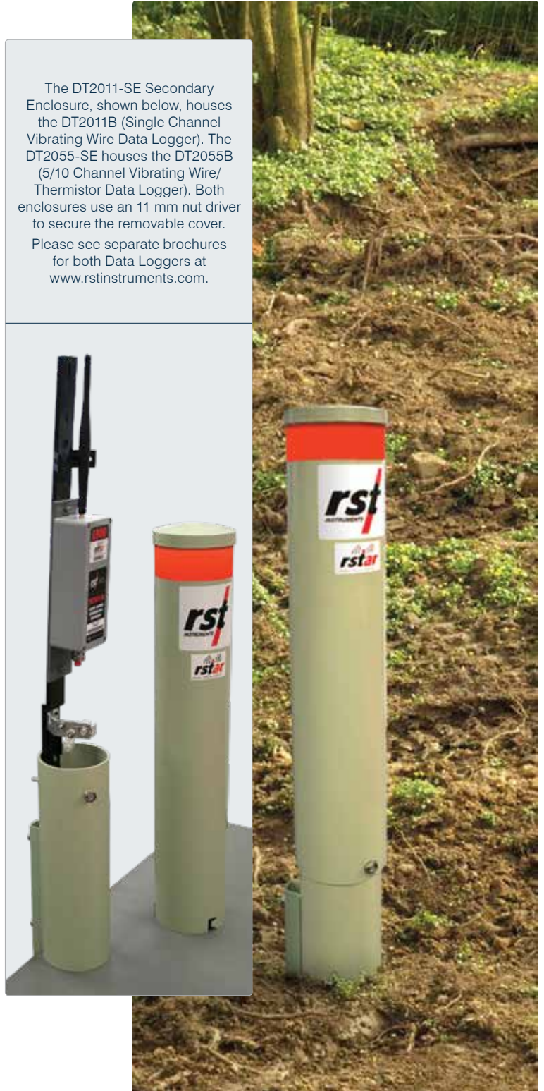
A DT2055B Ten Channel Data Logger shown housed in a DT-SE-1 Secondary Enclosure.
