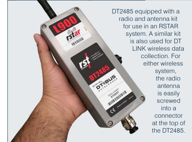
DT2485 equipped with a radio and antenna kit for use in an RSTAR system. A similar kit is also used for DT LINK wireless data collection. For either wireless system, the radio antenna is easily screwed into a connector at the top of the DT2485.
