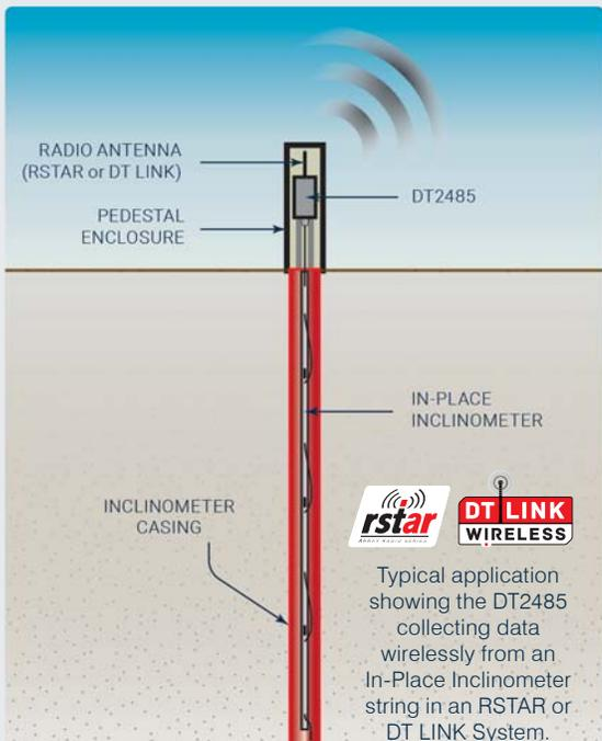
Typical application showing the DT2485 collecting data wirelessly from an In-Place Inclinator string in an RSTAR or DT LINK System.
