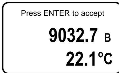
FIGURE 5-3 STORING A READING
