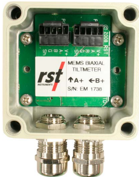
Figure 6 - Digital Bus Tiltmeter Electrical Connections
