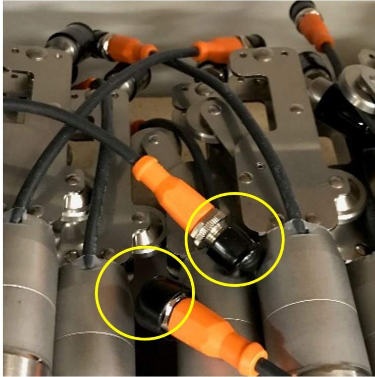
FIGURE 1-1 ENSURE PROTECTIVE CAPS ARE ALWAYS ON THE CONNECTORS
