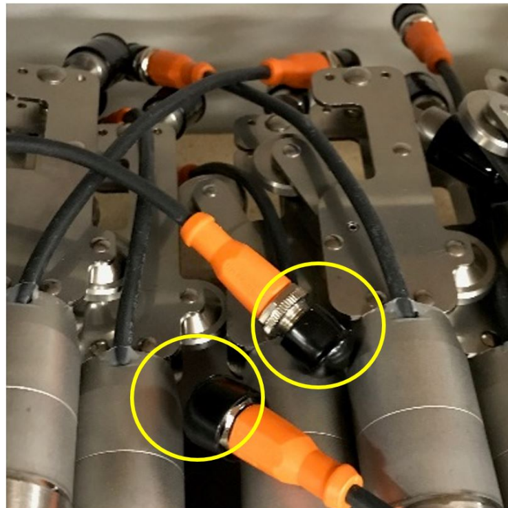
FIGURE 2-5 ENSURE PROTECTIVE CAPS ARE ALWAYS ON THE CONNECTORS
