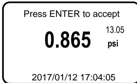
**Figure 21 – Storing a Reading**
