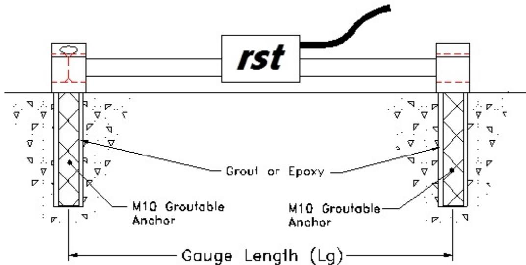
FIGURE 3-4 INSTALLATION ON CONCRETE USING GROUTABLE ANCHORS
