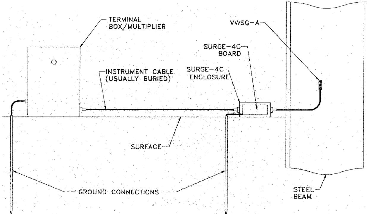
FIGURE 4-1 LIGHTNING PROTECTION SCHEME
