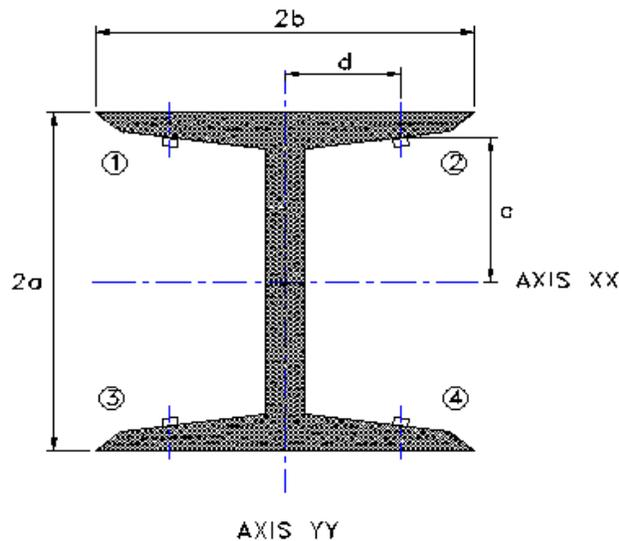
**FIGURE 6-11 STRAIN GAUGES MOUNTED ON FLANGES (NOT RECOMMENDED)**
