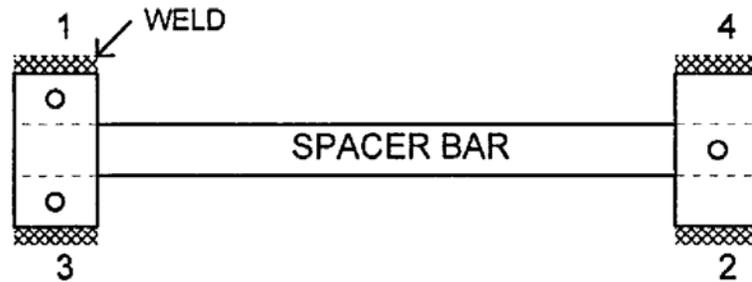
**FIGURE 3-3 WELDING SEQUENCE FOR THE MOUNTING BLOCKS**
